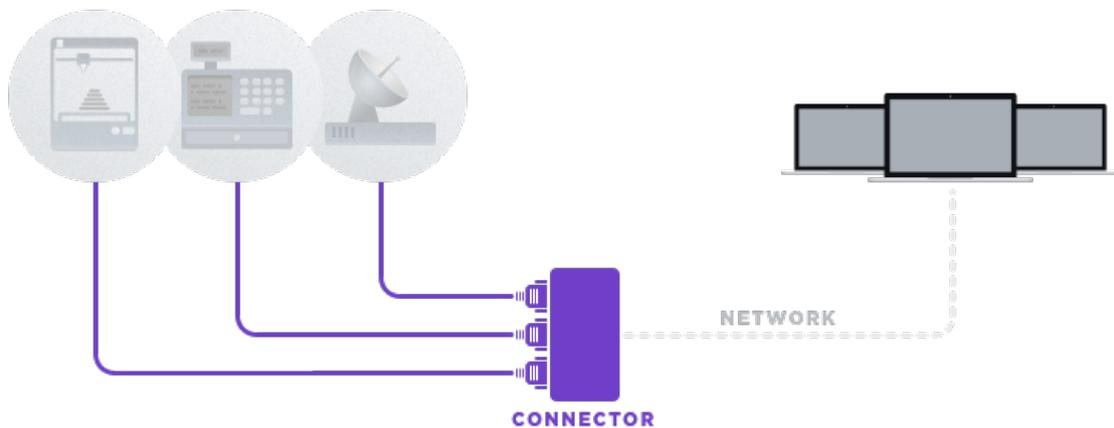
Considering the scale of production and physical remoteness of USB and serial devices, it's not always possible to establish a direct connection between required peripherals. In this case technical specialists have to resort to some hardware methods to share the peripherals over the network and access them remotely.
